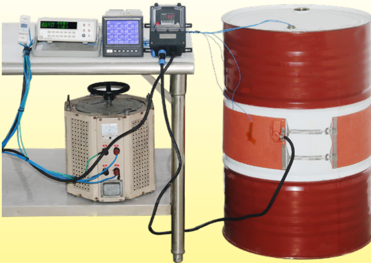
Variation in the temperature versus time of a 220-liter metal drum, filled with water, heated by a silicone heating belt 200mm wide, without thermal insulation, power 1500W (surface load 0.5W/cm 2 ).
