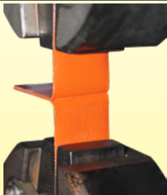
Vulcanized sample before decoupling test
