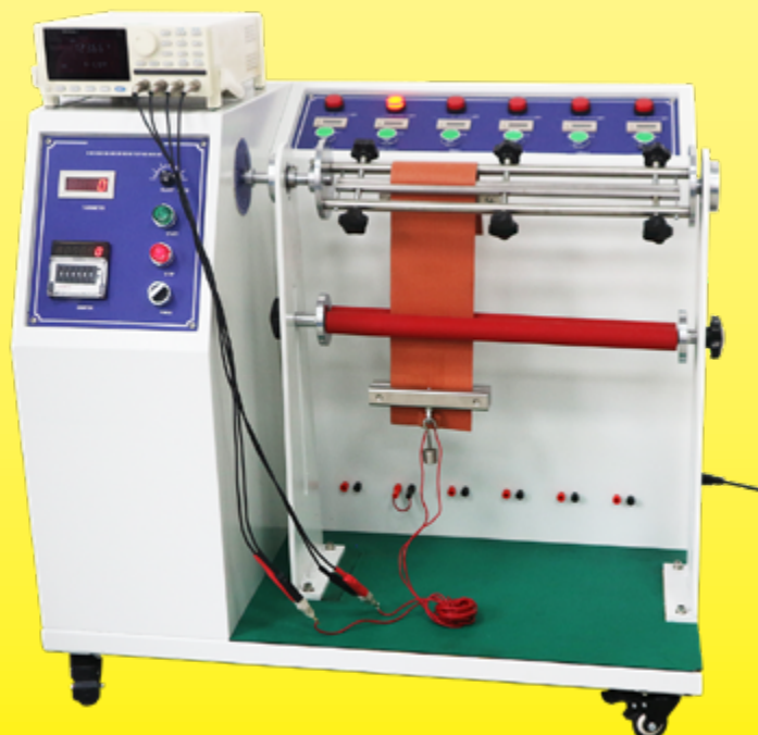
Flexible silicone heater during the flexion test
